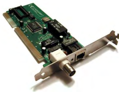
Gambar 6.9. Network Interface Card
