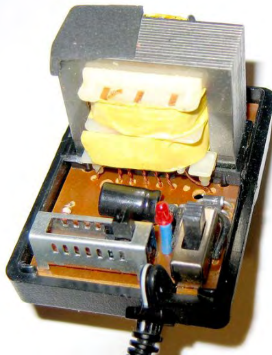
Gambar 4.10. Power Supply Unit.
